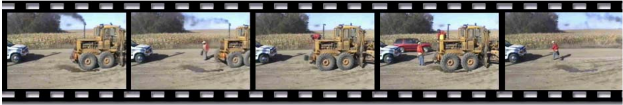
Figure 5. Video record taken by a camera programmed to respond to a proximity alarm.
